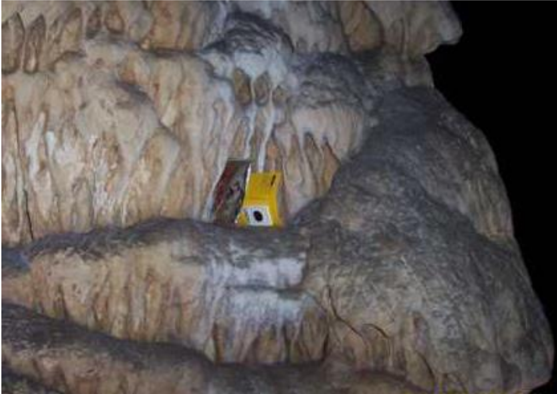
Fig. 5 - An etched track detector in place (Grotte di Toirano, Italy)
